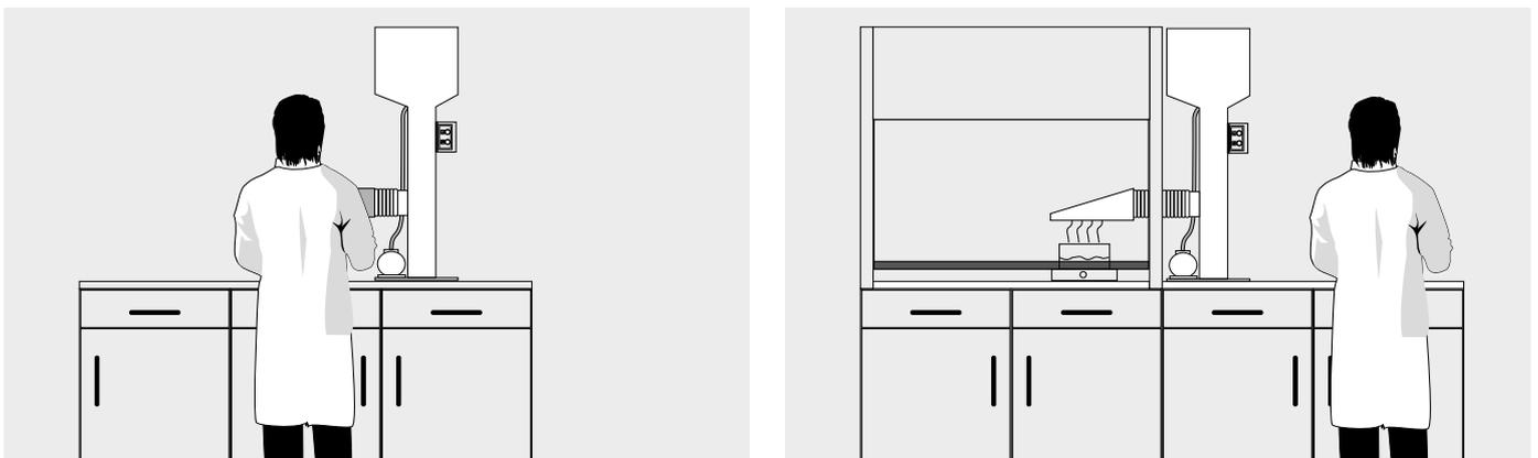
The fume scrubber C20 is flexible in its installation in the laboratory. Besides an installation on laboratory benches or on the floor it can be placed where the installation of a fixed scrubber is not possible due to restrictions of space. Please note that the unit must not be installed inside a fume cupboard.
